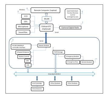
Figure 1: Structure diagram of the mobile platform and the external hardware system.
