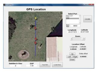
Figure 11: GPS Matlab GUI.
